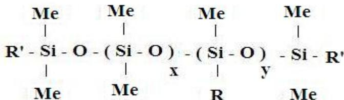
**Fig 4: Structure of Amino / Amido Silicones**
