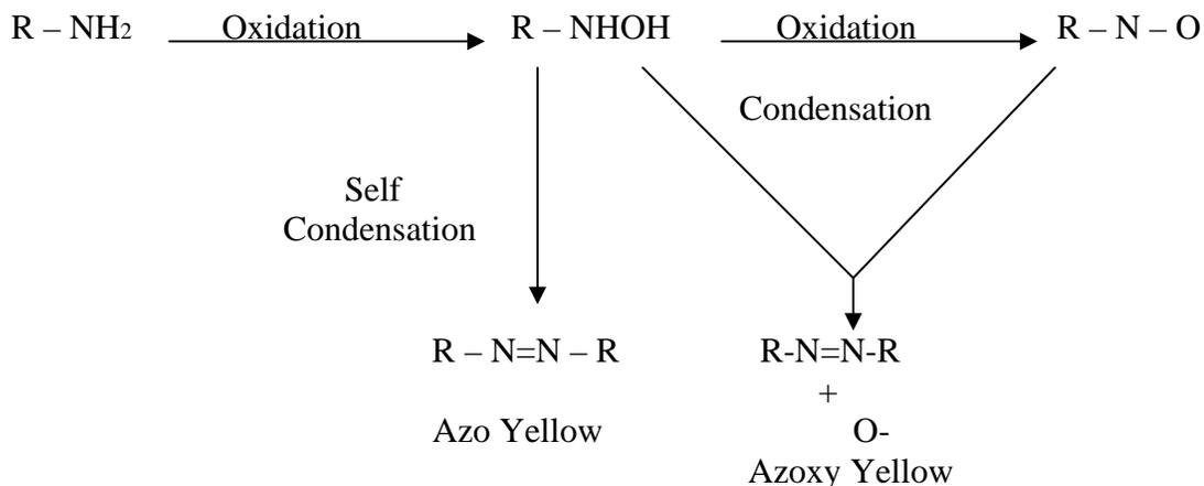
**Fig 5 : Mechanism of Amine Yellowing**
